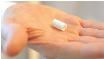
SUPPORT STRUCTURE: A 3-D–printed tracheal splint made of bioresorbable polycaprolactone is designed to fit around an infant’s collapsing airway. COURTESY OF JENNIFER LEWIS
