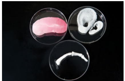
BUILDING BODY PARTS: Anthony Atala has printed a kidney prototype (left) and biomaterial scaffolds for growing new ears (top right) and finger bones (bottom).
