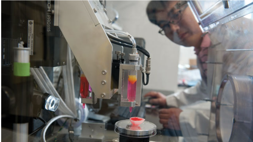
RENAL RECONSTRUCTION: Wake Forest postdoctoral fellow Hyun-Wook Kang operates a 3-D printer that is making a kidney prototype with cells and biomaterials.
