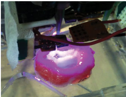
FAB MACHINE: University of Nottingham tissue engineer Kevin Shakesheff uses a Fab@Home printer (top) to engineer bone. Others have used the open-source printer for printing heart valves (bottom), ears, and more. COURTESY OF THE LABORATORY OF JONATHAN BUTCHER, CORNELL UNIVERSITY
