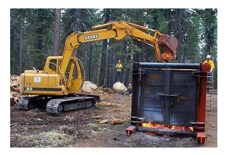
Figure 16. Air curtain burner.
