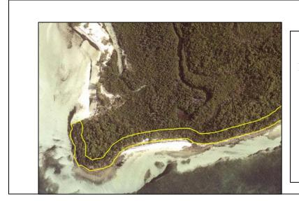
Example of coastal buffer zone delineation along low energy rocky shore of the BBC property – this buffer zone is incorporated into the planning process, and delineated with protective fencing during construction
