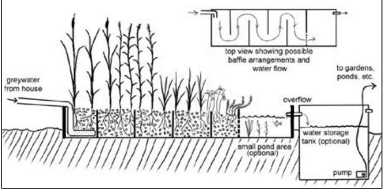
Figure 17. Schematic diagram of a phytoremediation wetland. Copyright Lawrence Fields. Photograph by Lawrence Fields.
